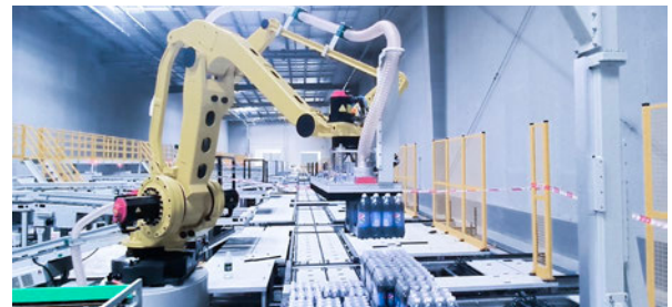
Vision-Guided Depalletizing of Shrink-Wrapped Bottles
