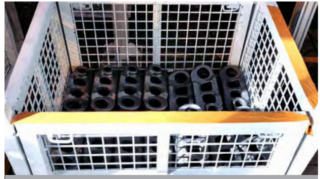
Severe stacking of workpieces, accompanied by typical ambient light interference in the workshop, and deep baskets.
