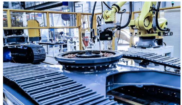
Vision-Guided Grease Applying for Swing Bearings
