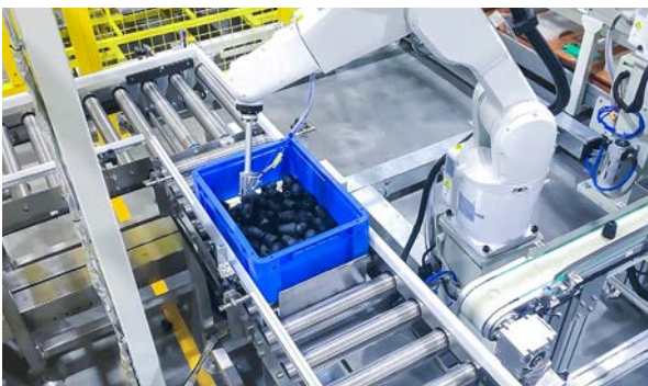
Vision-Guided Bin Picking of AC Foot Pads
