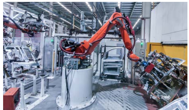
Vision-Guided Car Door Inner Panel Picking
